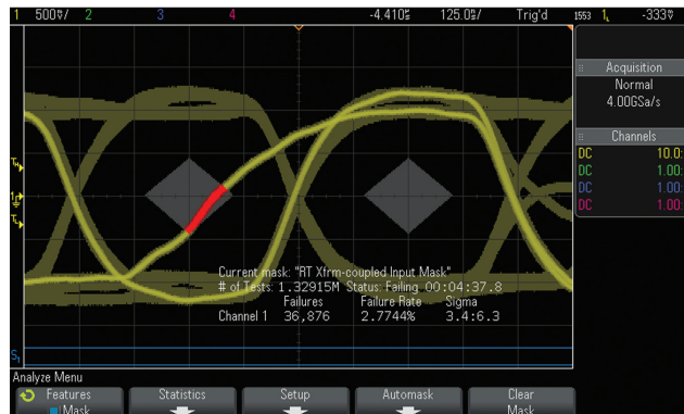
Figure 3. MIL-STD 1553 eye-diagram mask test on Command Words received at a specific remote terminal.
